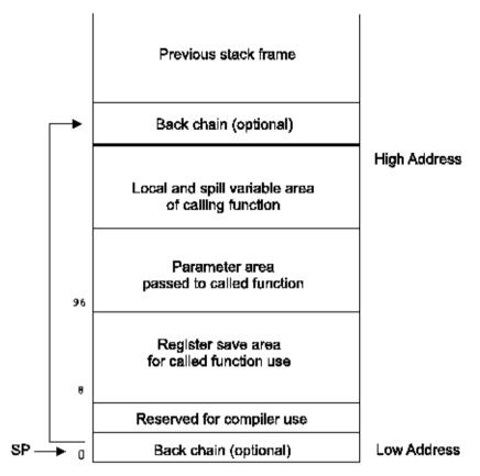
Figure 1-15. Standard stack frame
