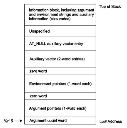
Figure 1-22. Initial Process Stack
